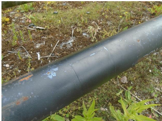
Image 4 4in pipe loop – East End PermaTool - Bonded Magneto strip
